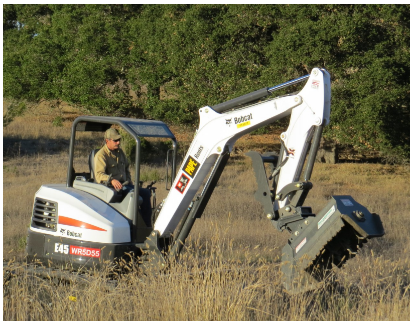
Figure 6. Vegetation masticator, Monterey County.
